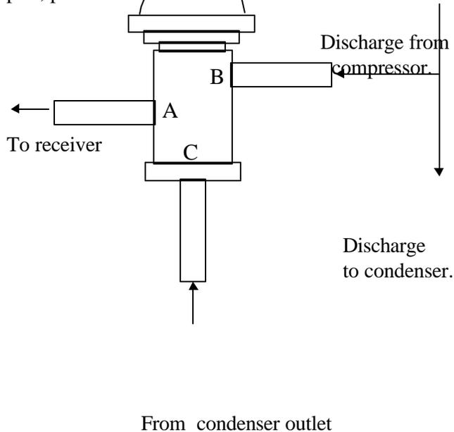
The headmaster will direct the flow of either discharge gas or liquid refrigerant to the receiver. The valve can throttle or modulate open and closed to maintain proper high side receiver pressure. This throttling action allows the system to maintain a solid column of liquid refrigerant to the TXV refrigerant control.
